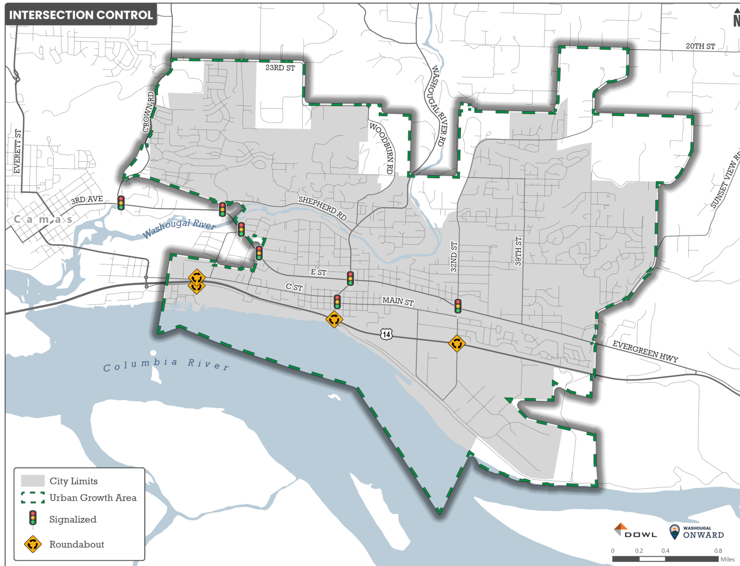
Figure 19. Existing Traffic Control at Signalized and Roundabout Intersections in Washougal
