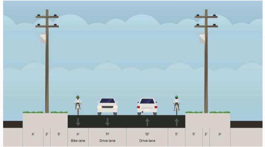
EXISTING 39th Street Roadway Section NTS
