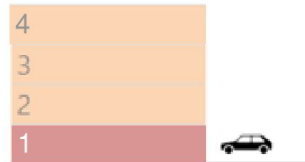
surface parking Type V-A wood frame construction
