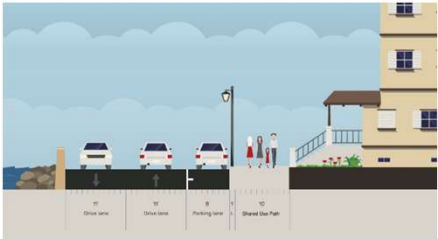
Proposed Typical Roadway Section
