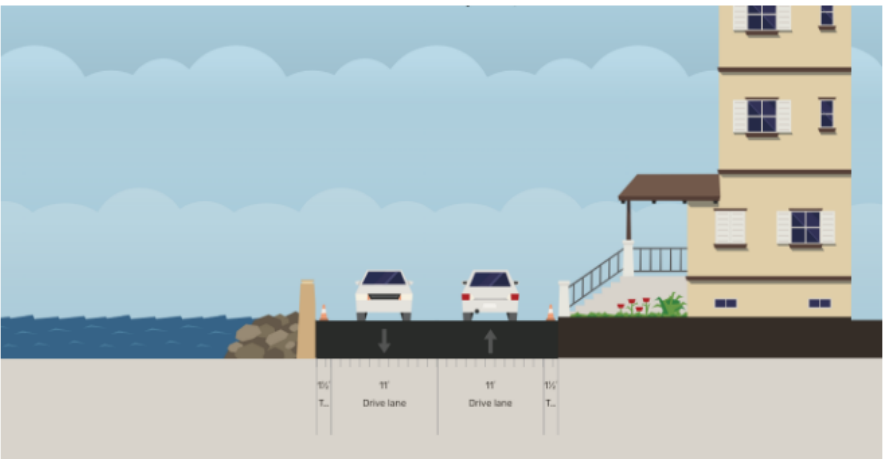
Existing Typical Roadway Section
