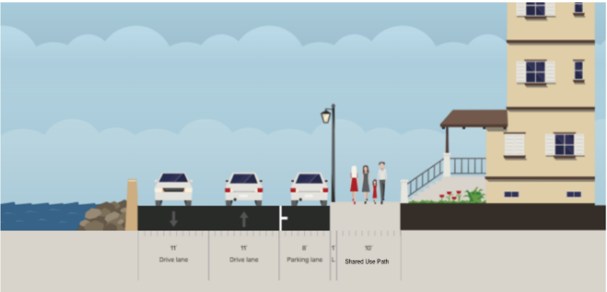
Proposed Typical Roadway Section
